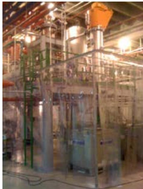
Figure 41. a) 35,000 Gal. Hydrolysis Reactors and b) 10T/D Pre-treatment Skid [ICM]
